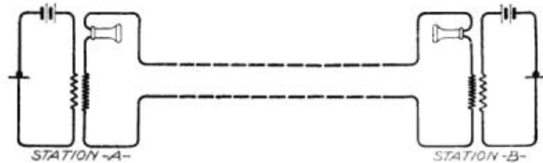
Fig. 126. Local-Battery Stations with Metallic Circuit
