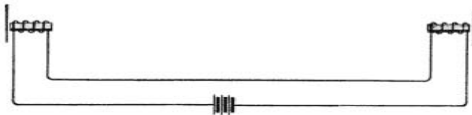
Fig. 3. Magneto Telephones without Permanent Magnets
