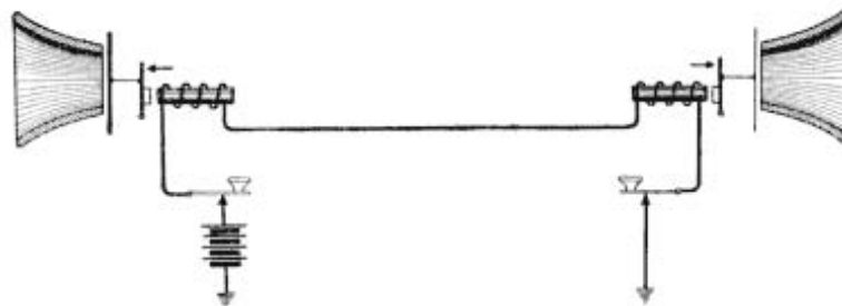
Fig. 6. Telegraph Equipment Converted into Telephone Equipment
