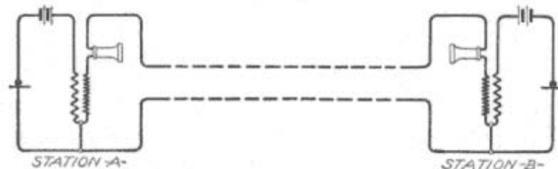
Fig. 127. Local-Battery Stations with Metallic Circuit
